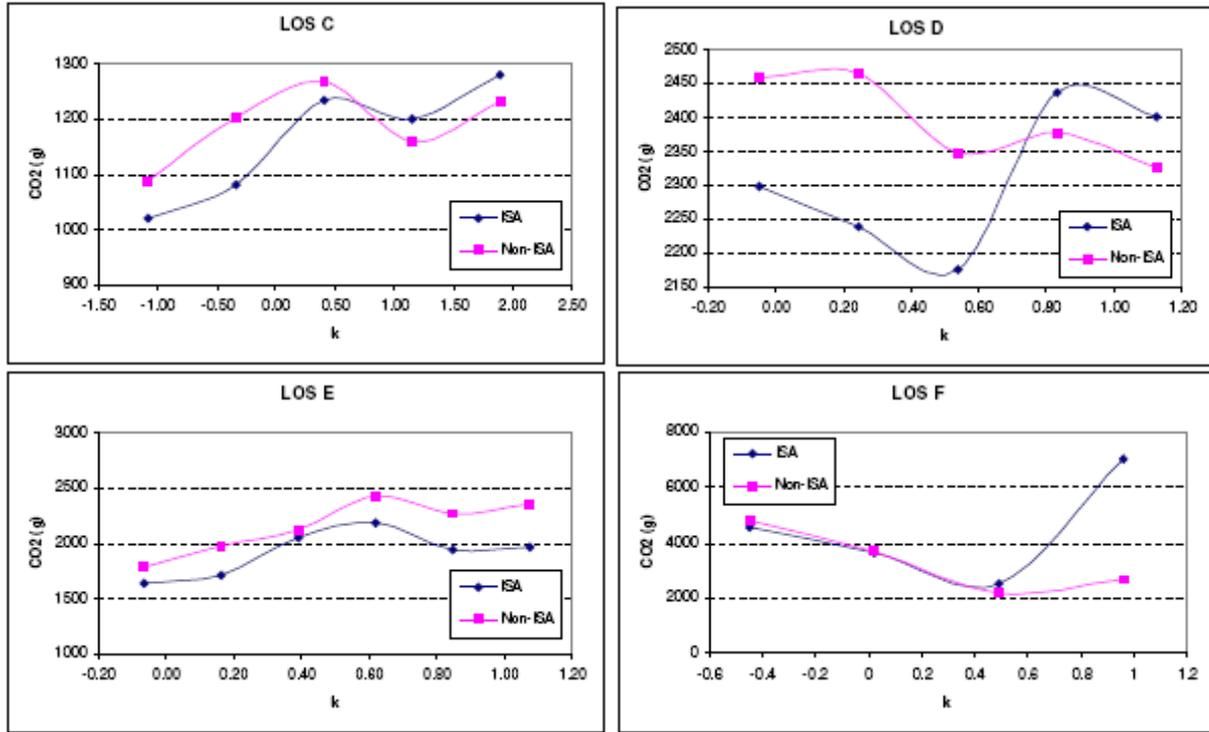
Figure5: Effect of control speeds on CO<sub>2</sub> under different levels of congestion.
